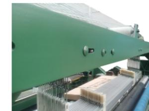
Thick 14cm girder with long screw trough for flexible adjustment
