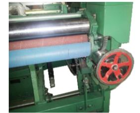
Bearing embedded continuous take-up mechanism
